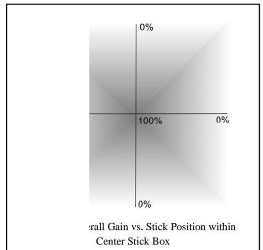
Gain Knob to 0%. Bringing the stick back to center will bring the Overall Gain back to its original value, set either by the "Stabilizer Overall Gain" parameter or by the Aux2 servo input as explained in the section "Stabilization "Master Gain" Knob."
