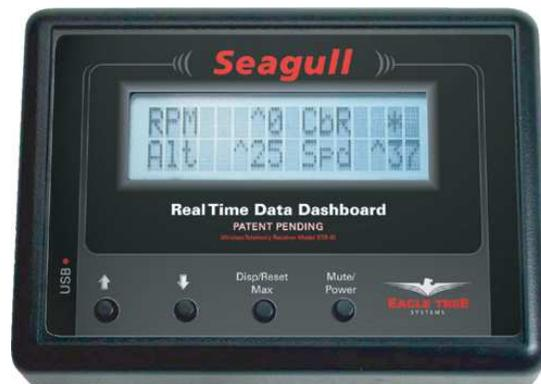
**USB Connection:** The USB cable supplied with your Recorder connects to the Dashboard at this port. Note that the RED wire of the USB cable goes up, as shown by the red dot above “USB” on the Dashboard label. **NOTE: If you have a 9V battery in the Dashboard, the Dashboard must be powered on before connecting to USB.**
