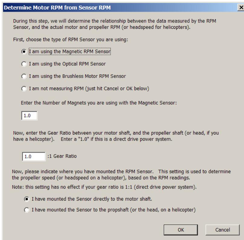
If you have a magnetic RPM sensor, enter the number of times your motor turns with each rotation of the magnets as described in this dialog box. If you have an optical or brushless RPM sensor, please see the instructions included with that sensor.
